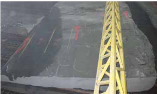
Wire cut blocks, up to 5 tonnes in weight, are carefully removed and inspected by "Markers" specially trained experts, who identify where the extracted blocks should be sawn and what the ultimate, optimised slate dimension will be. This stage is not common in other slate producing regions.
