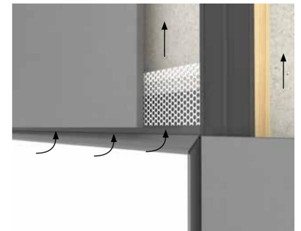
A horizontal free ventilation opening must be maintained above windows and doors as well. This ventilation gap must be at least 10mm wide. If steel, aluminium or plastic perforated profiles are used, a ventilation area opening of minimum 100cm<sup>2</sup> per meter is required. The opening at the base is also used to drain moisture that has entered the facade.
