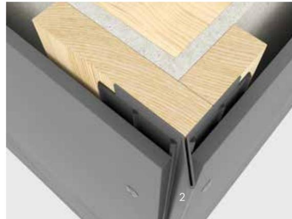
Cembrit External Corner Peak can also be used for 90° external corner constructions. It is installed in the same way as Cembrit External Corner Small, using clout nails. The distance from the inside edge of the facade boards to the profile should be a minimum 2mm.
