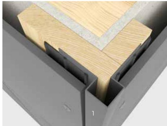
Cembrit External Corner Small is used for 90° external corner constructions, to a secure finishing detail. The profile is fixed using clout nails at 400-500mm centres through pre-drilled Ø4mm holes. Facade boards will help to hold the profile in place. There should be a minimum 4mm gap between the board edge and the profile.
