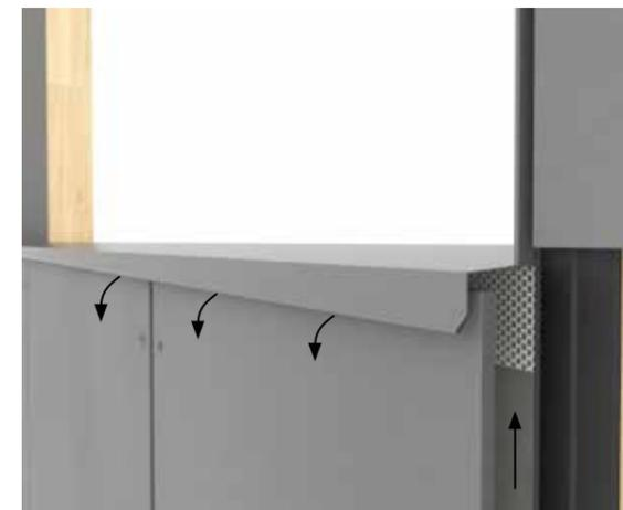
A horizontal ventilation opening of minimum 10mm or equivalent to 100cm<sup>2</sup> per meter should be maintained beneath windows or other openings where a sill is used. This ventilation gap is usually formed between the top edge of the facade boards and the bottom edge of the sill. It is recommended that the sill projects a minimum of 30mm beyond the front of the facade. This ensures that the water running from the sill does not enter the structure.
