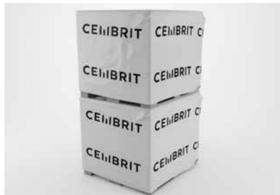
Only two pallets must be stacked on top of each other. Make sure they are positioned so they stand securely and stable.
