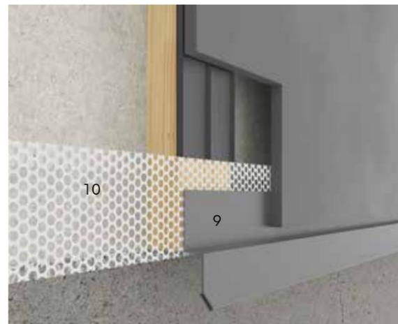
Cembrit Drip Small is used to drain water away from the supporting structure or where neat detailing is required at the foot of the facade. The profile can be used in conjunction with Cembrit Ventilated Profile to ensure that insects and vermin or similar cannot enter the cavity behind the facade boards. There should be a minimum 4mm gap between the board edge and the profile.
