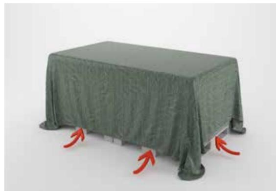
Replace the plastic with a tarpaulin. It is very important that there is ventilation all around the tarpaulin and also on top of the pallet under the tarpaulin. This is done to make sure that condensation is reduced as much as possible.
