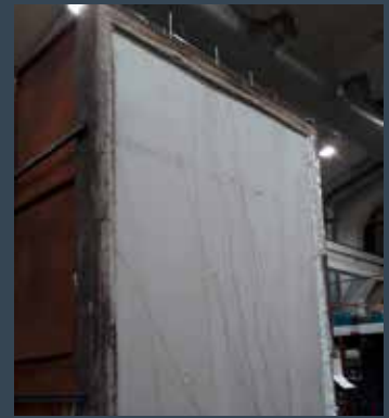
Windstopper Extreme fire test at VTT
